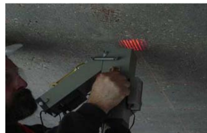
b) Roughness Detection by Laser Profilometer
