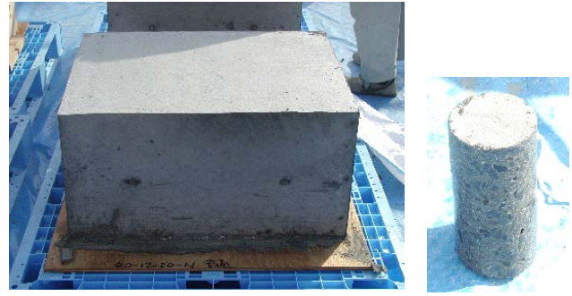
Fig.8 Alkali-aggregate reaction and velocity ratio Fig.9 Standard concrete block test specimen and sampling core
