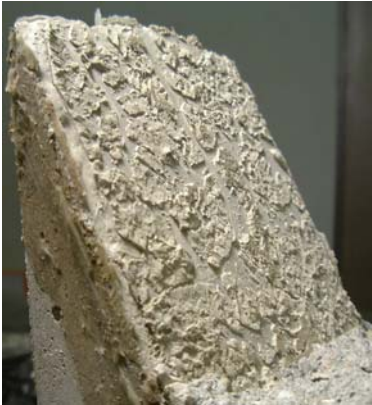
Fig.8 Fracture surface in the crack repair division.
