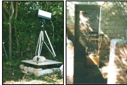
Figure 10 – SLDV mounted on isolation platform and road plate compactor used to excite the building.
