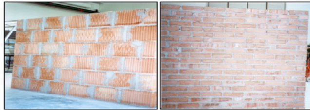
Figure 5 – Sample brick walls (Poroton bricks, left, normal bricks, right), walls 1.8 (L) x 1.5 (H) x 0.25 (W) m.
