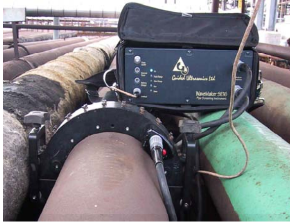
Fig 1. Solid transducer ring for 8 inch pipe and battery powered test instrument on site.
