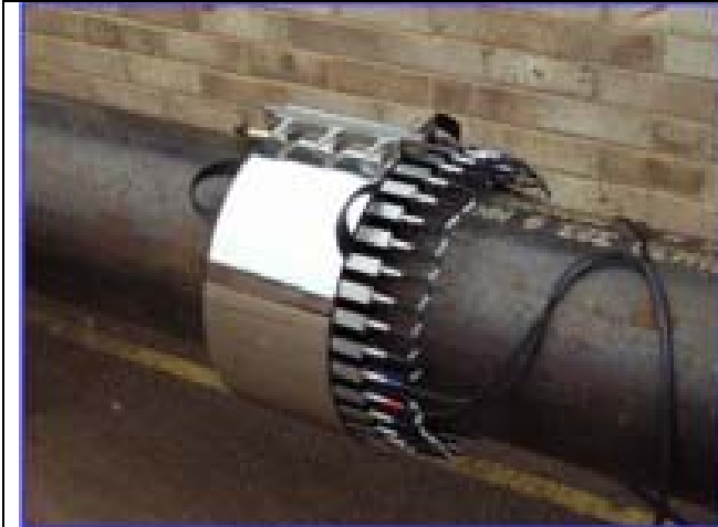
Figure 2. 14-inch guided wave inspection collar. Individual transducer modules can be seen on the right side of the collar in the picture. Modules are mounted in a pneumatic bladder covered by a steel sleeve. Inflating the bladder applies uniform pressure on the transducers. There are 120 transducers in the collar shown.
