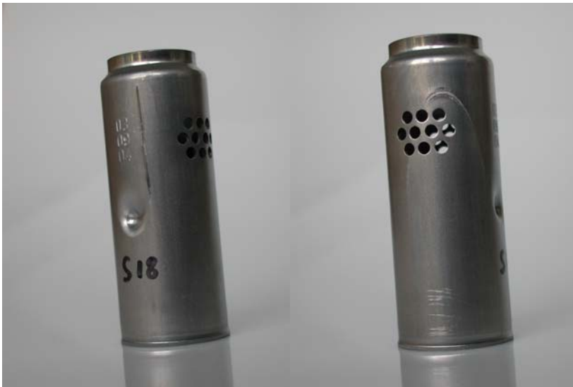
Fig. 7: Airbag tubes with crack (left) and crinkle (right)
