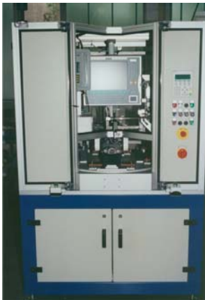
Figure 5. Integrated test bench with eddy current and resonance testing for brake components
