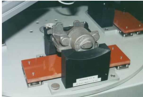
Figure 5. Integrated test bench with eddy current and resonance testing for brake components
