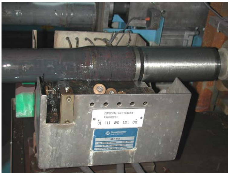
Fig. 4: Inspection of upset ends with REP-VIS
