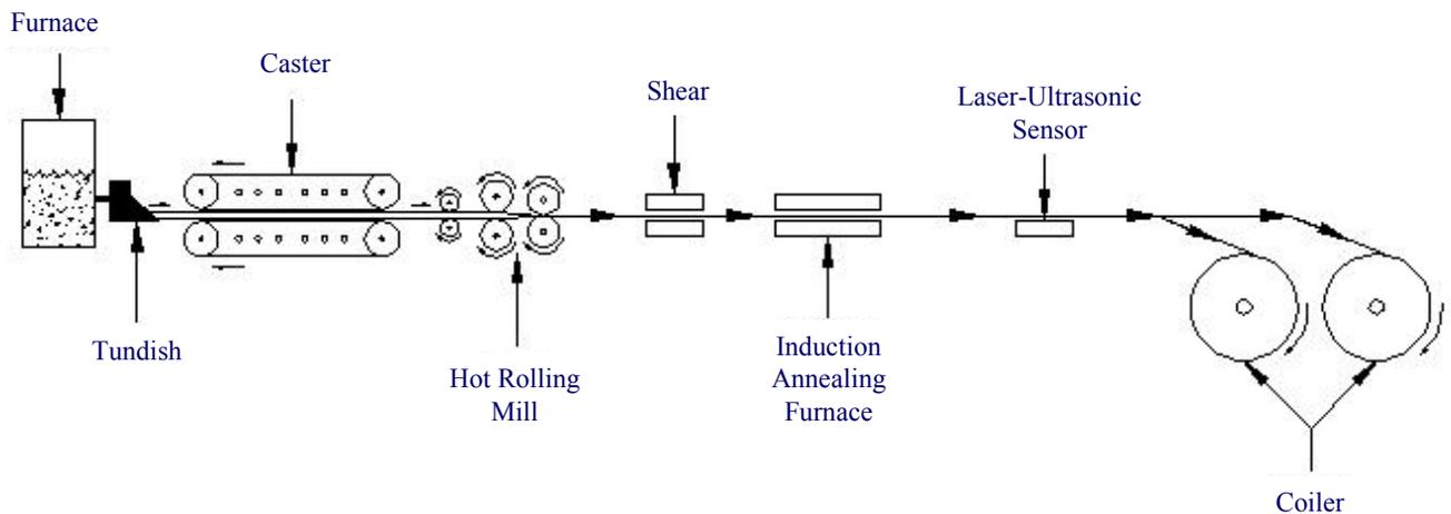
Figure 1. Schematics of the inline annealing process, including inline laser-ultrasonic monitoring of recrystallization.
