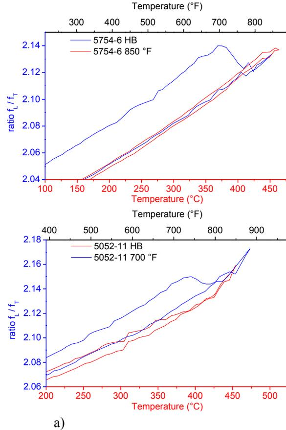
Figure 2. Temperature dependence of the ratio of the longitudinal to transverse sound velocity during heating and cooling at a rate of 1 °C/s for, a) two samples of AA5754 and, b) two samples of AA5052. The designation HB (blue line) refers to hot band samples that are not fully annealed, while the temperature designation (850 °F or 700 °F, red line) refers to the approximate maximum temperature the inline annealed samples reached during inline annealing.
