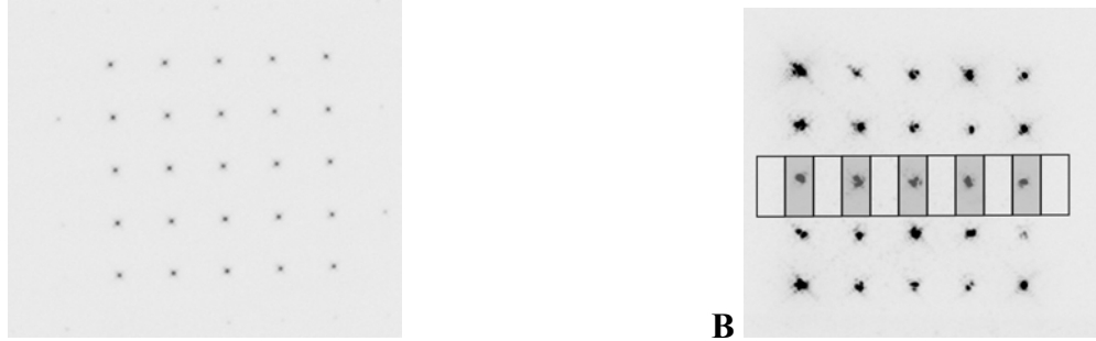
Fig. 2 : Image of the array of spots in the target plane (A) and in the detector plane (B) with the dimensions and the position of the photodiode line indicated.
