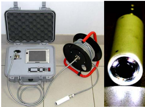
Fig. 9. TV-endoscope with fibre glass illuminator at the working tip
