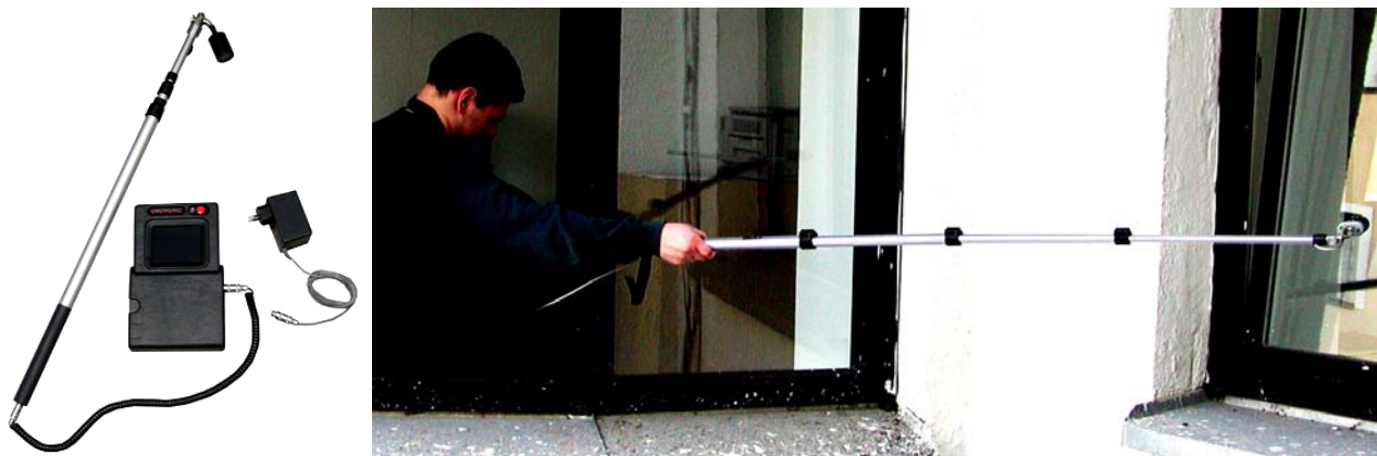
Fig. 11. TV- device “Poisk-TV” for observation of difficult to access areas
