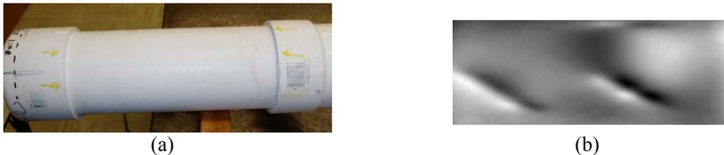
Fig. 7. NDT of a plastic PVC pipe with two flaws inside loaded by an internal pressure change of 0.02 Mpa; (a) live image, (b) measuring result
