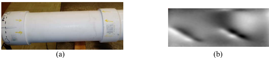
Fig. 7. NDT of a plastic PVC pipe with two flaws inside loaded by an internal pressure change of 0.02 Mpa; (a) live image, (b) measuring result
