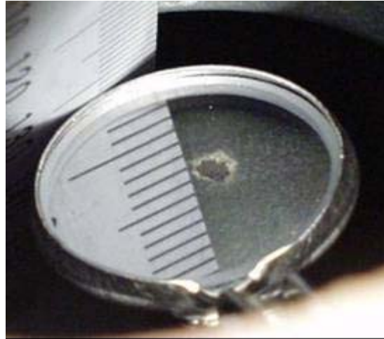
Figure 2. Chip in throat of PRCS thruster.
