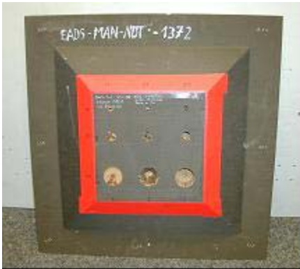
Fig. 6: Results of performed test on fuselage out of CFRP monolithic structure Next tests were carried out on test samples of CFRP-H/C-structure (fig. 7a). In this test samples debondings of the H/C core are simulated by holes of various depths. It is shown that the holes which are penetrating the complete honeycomb core pointed out very clearly (fig. 7b). The other holes are difficult to recognize. Additionally many defect indications distribute on the entire testing area are shown. After a X-ray examination (fig. 7c) it was determined that there is an accumulation of resin within the H/C cores.
