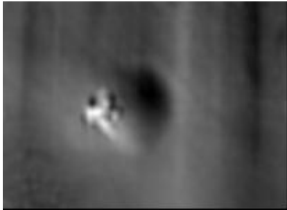
Fig. 6: Results of performed test on fuselage out of CFRP monolithic structure Next tests were carried out on test samples of CFRP-H/C-structure (fig. 7a). In this test samples debondings of the H/C core are simulated by holes of various depths. It is shown that the holes which are penetrating the complete honeycomb core pointed out very clearly (fig. 7b). The other holes are difficult to recognize. Additionally many defect indications distribute on the entire testing area are shown. After a X-ray examination (fig. 7c) it was determined that there is an accumulation of resin within the H/C cores.
