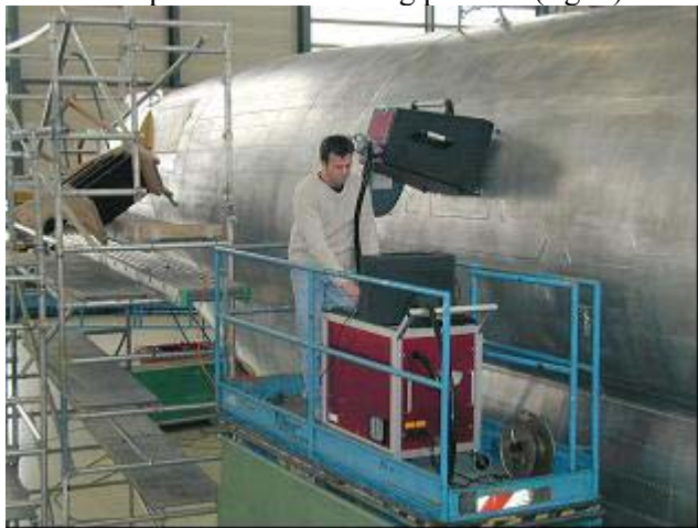
Fig.3: First performed tests on a aircraft fuselage with aluminium honeycomb structure
