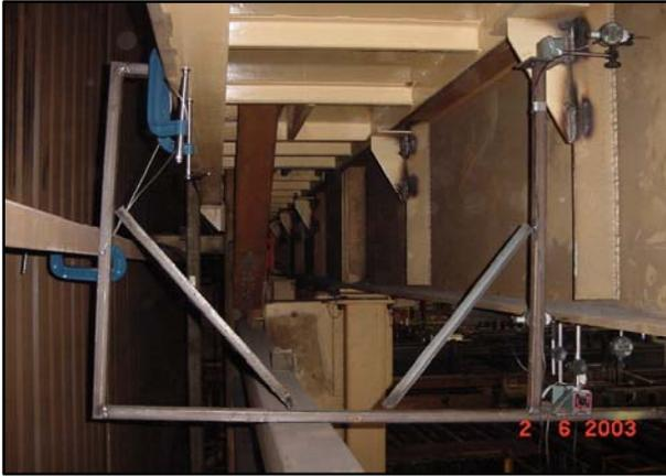
Picture No 2: Set-up for digital indicators installation
