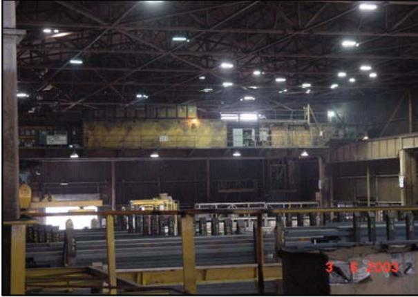
Picture No 3: 22 tons heavy service overhead crane
