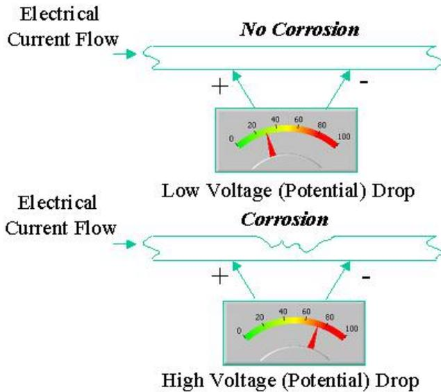
Figure 3: Schematic demonstration of the resistance corrosion measurement
