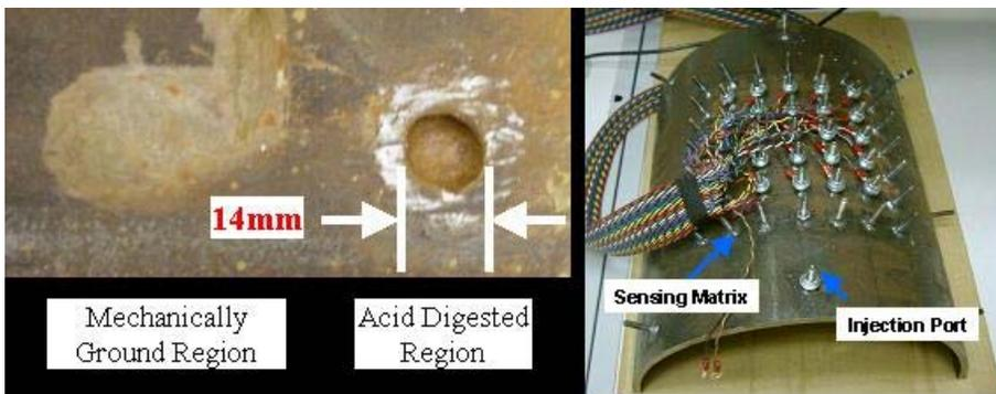
Figure 5: Test sample used for simulated corrosion tests
