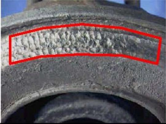
Figure 2: Pump component showing naphthenic acid corrosion (Outlined in red)
