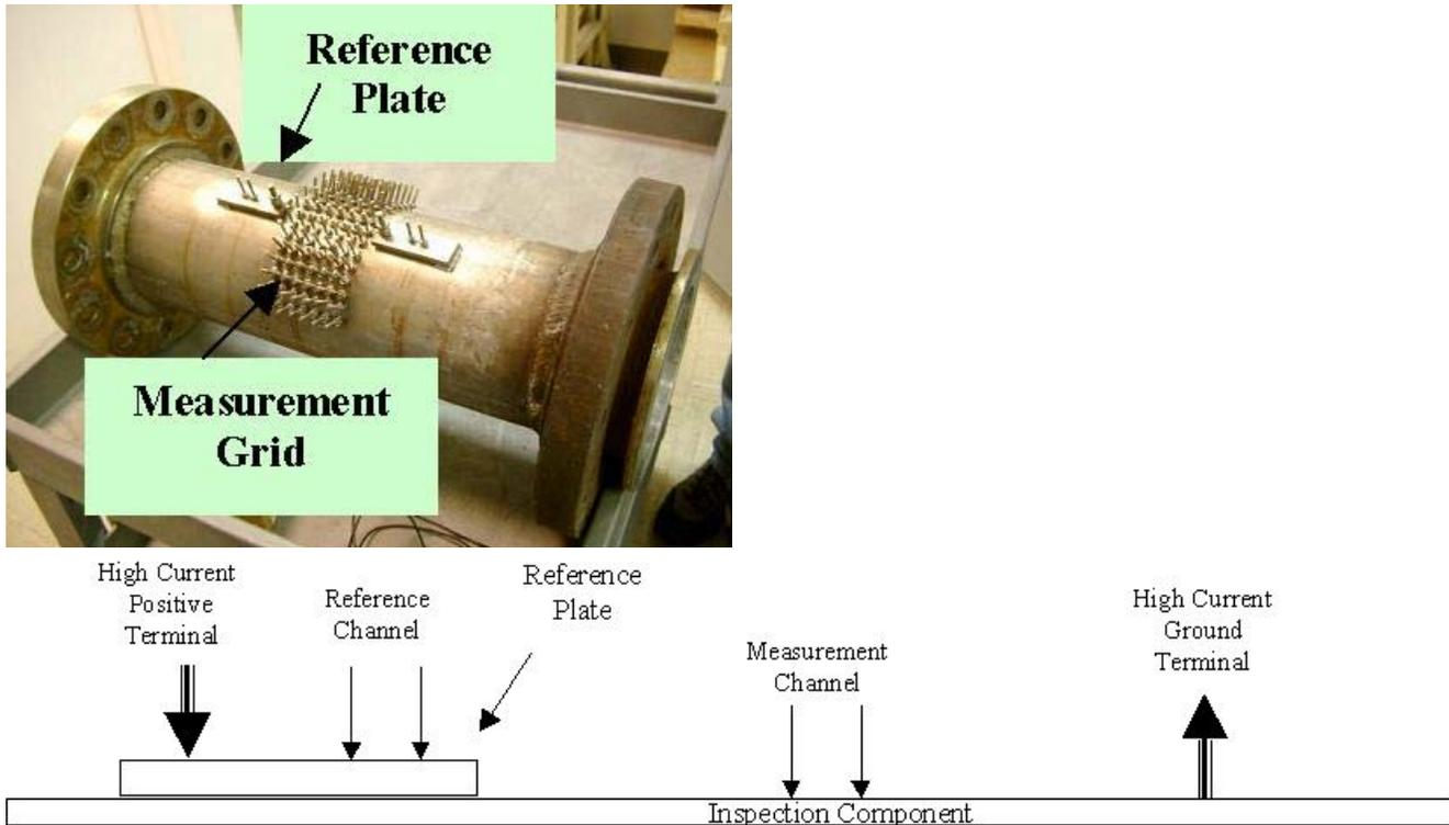
Figure 4: Typical field test setup
