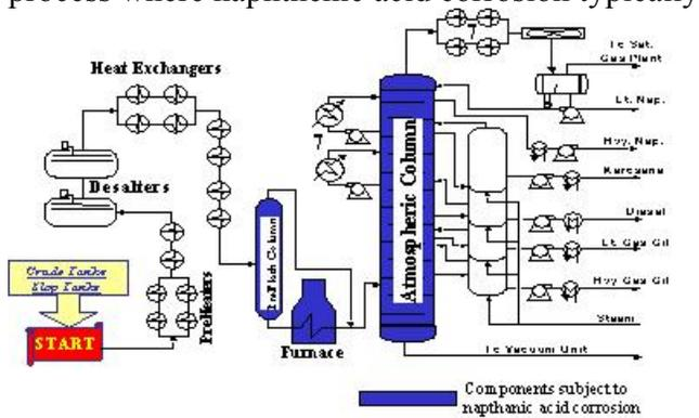
Figure 1: Crude oil refinery “Crude Unit”. Blue indicates components subject to naphthenic acid corrosion. [2]
