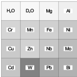
Figures 2 (left) and 3 (right): Transmission properties for X-rays, gamma-rays, thermal and 1.7 MeV neutrons for different materials. In the individual areas the charge number is increasing from top left to bottom right, i.e. the densest material is located at bottom right. The darker an area the less its transmission.
