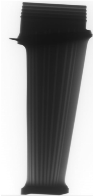
Fig.1 Inspection image of turbine blade
