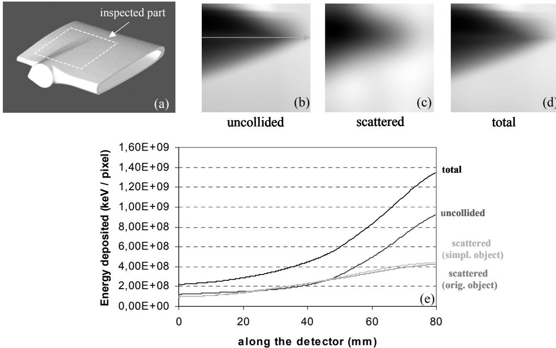
**Figure 7 : Application example. Test part geometry (a), simulated uncollided (b), scattered (c) and total flux images (d) and profiles along a horizontal axis (e) of all images, included scattered images computed with the original complex object (114 300 facets) and the simplified object (798 facets).**
