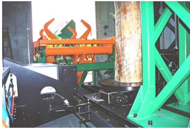
Figure 2. Interior view of the CT scanner bay with a log loaded and ready for scanning.
