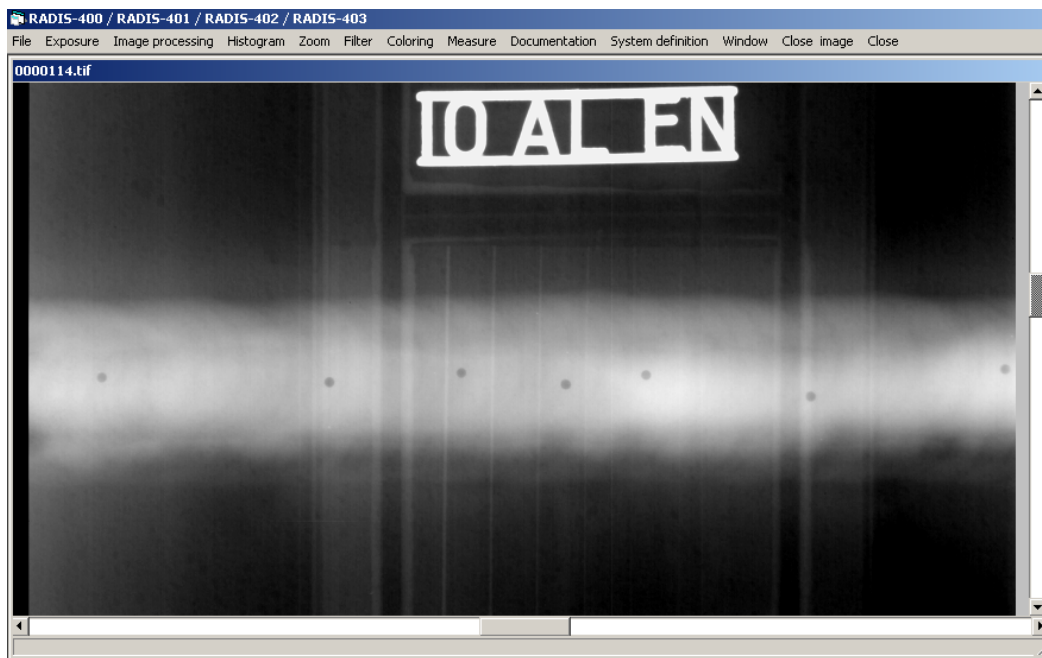
Fig. 12: Digital radiograph of a circumferential weld (Aluminium 400x18 mm, single wall exposure, 60 kV, 30s, 1mm drill holes, 1mm deep, zoom 250%)
