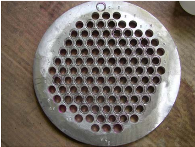
Fig. 13: Tube to bottom welds in a heat exchanger bottom
