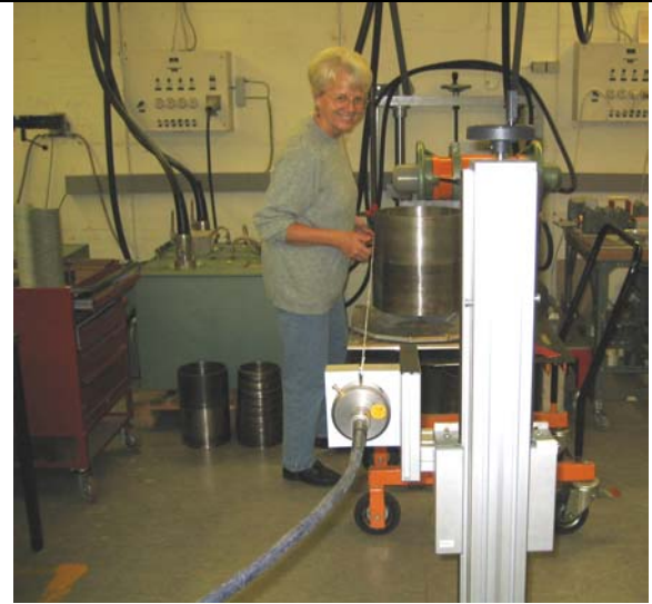
Fig. 5: Alignment of the radiation source (Co 60) for the tangential projection technique. Behind the 12 inch pipe is the film cassette. The pipe sits on a turn table for easy positioning of the different holes in relation to the film.
