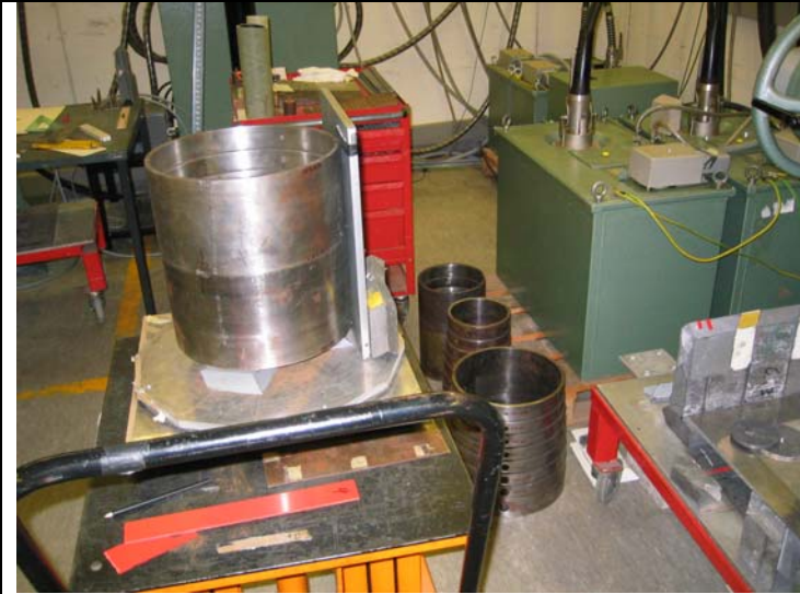
Fig. 4: The finalized test specimen at BAM (8 inch steel pipe with inner and outer wall thickness steps separated for better handling, one 12 inch pipe at exposure arrangement ready for inspection, the other 12 inch pipe with outer wall thickness steps at the floor)
