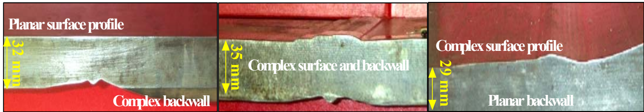
Figure 2: Examples of machined mock-up of complex surface and/or backwall dedicated to experimental validation of contact inspection simulations
