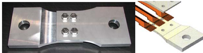
(d) Four-hole specimen and a schematic with 3 linear MWM-Arrays embedded between layers.
