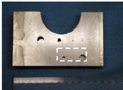
Figure 6: Mg/Al testpiece with flat bottom holes of diameters 10, 5, 1 and 0.5 mm. The dashed rectangle indicates the inspected area for SAFT processing.
