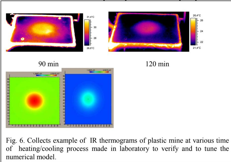
Fig. 6. Collects example of IR thermograms of plastic mine at various time of heating/cooling process made in laboratory to verify and to tune the numerical model.
