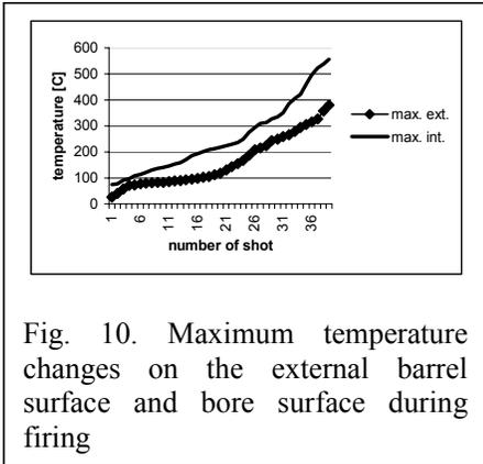
Fig. 10. Maximum temperature changes on the external barrel surface and bore surface during firing
