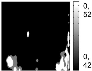
Fig.7. Map of thermal contrasts during 3 June 98 and scaled for mine at 2.5 cm depth ( placed at left bottom corner)
