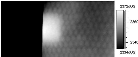
Fig.3. Phase image ( $f = 0.03$  Hz) composite with defect in form of separation of several cells from cover.
