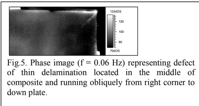
Fig.5. Phase image ( $f = 0.06$  Hz) representing defect of thin delamination located in the middle of composite and running obliquely from right corner to down plate.
