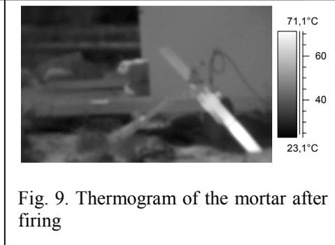
Fig. 9. Thermogram of the mortar after firing
