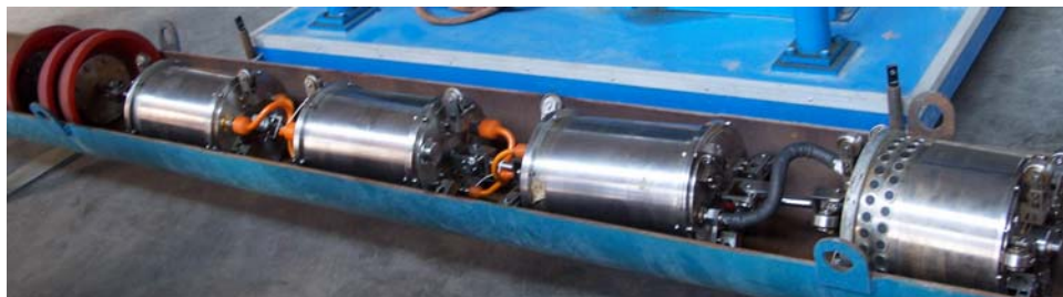
Figure 1 the ultrasonic inspection pig
