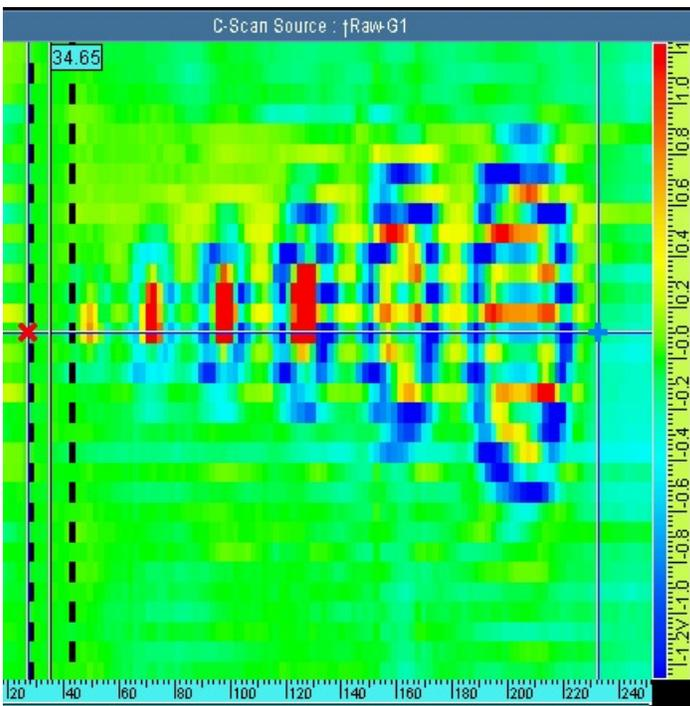
3b. Traditional modular eddy current array output for 4<sup>th</sup> layer defects (1mm material loss plate below 3 1mm layers)
