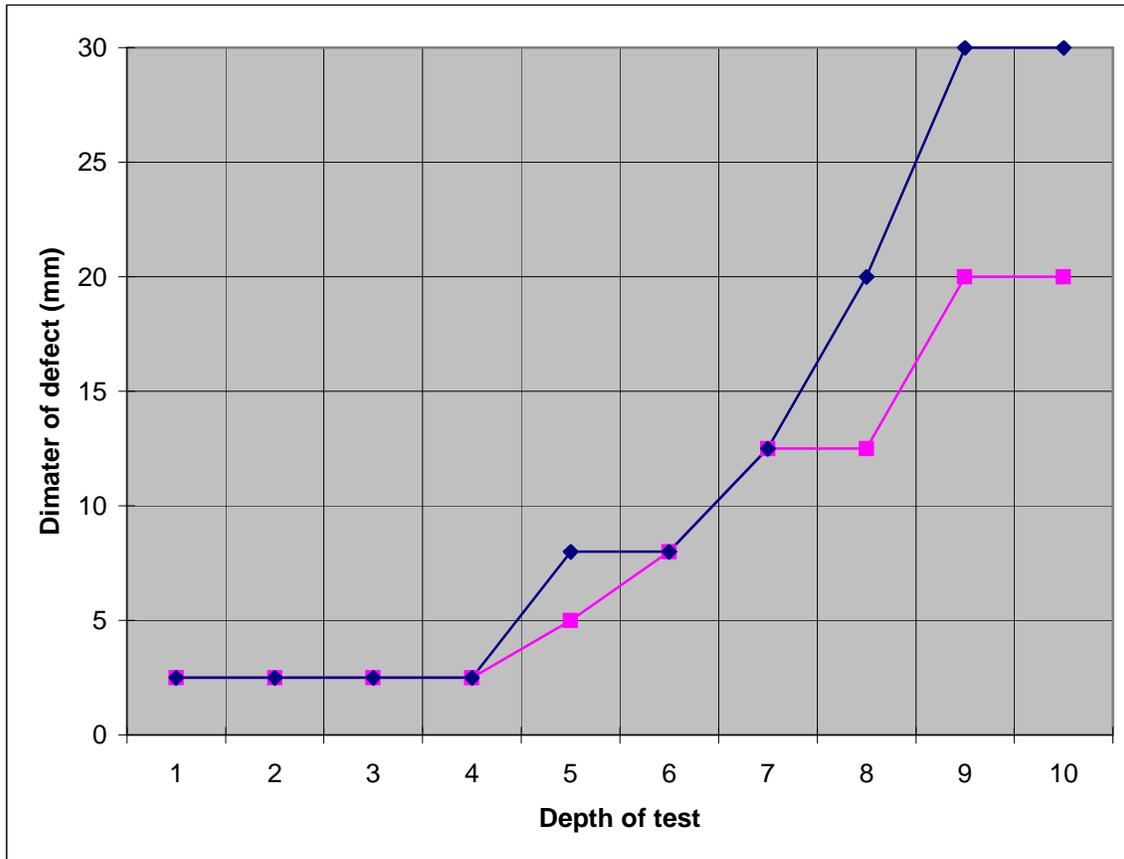
Figure 4. Blue = Traditional modular eddy current; Pink = Pulsec™ Pulsed eddy current
