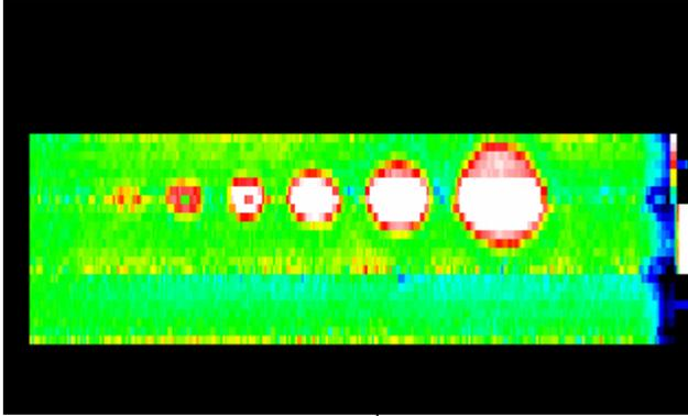
3a. Pulsec™ image for 4<sup>th</sup> layer defects (1mm material loss plate below 3 1mm layers)
