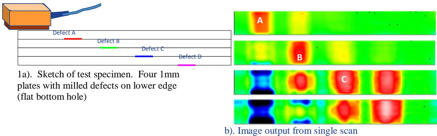
1a). Sketch of test specimen. Four 1mm plates with milled defects on lower edge (flat bottom hole)
