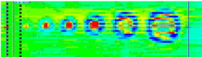
3c. Traditional modular eddy current array output for 4<sup>th</sup> layer defects (1mm material loss plate below 3 1mm layers). Image rescaled to 1:1 aspect ratio.
