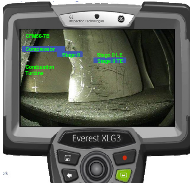
Figure 2; Sample inspection list selection screen as seen by operator on the VideoProbe®
