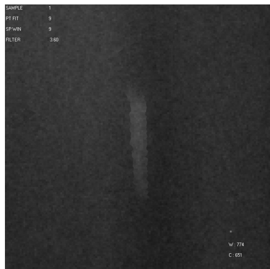
Figure 21: 7x ROI of the 'bubble' defect 'after' enhancement.
