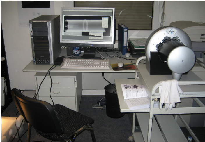
Fig. 1: Duerr HD-CR 35 imaging plate scanner system (right) equipped with a personal computer (left) for data storage and image evaluation on a high contrast display.
