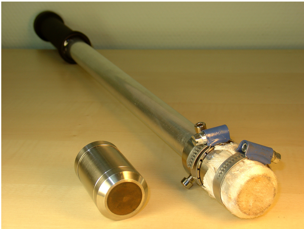
Fig. 4. EMA transducer for testing the hot objects: left – without heat protection; right – on the handle with heat protection from fiberglass.
