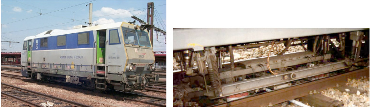
Figure 1. SNCF ultrasonic inspection train (left), ultrasonic probes support (right)
