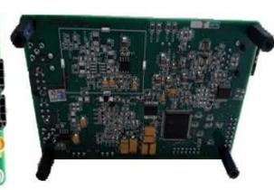
**Fig.5.** 2 MHz Transceiver Board
