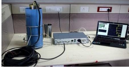
**Fig.9.**Ultrasonic Diameter Measuring System
