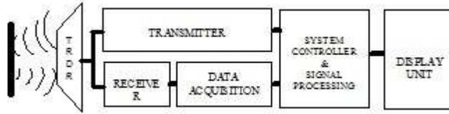
**Fig.1.** Block diagram of distance measurement system
