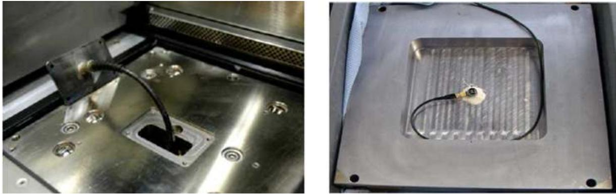
Figure 2. Ultrasonic probe arrangement underneath the build-platform.
