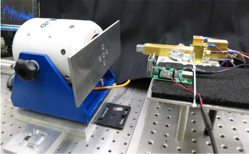
Figure 4: Harmonic vibration measurements using a shaker system and the two transceiver systems.
