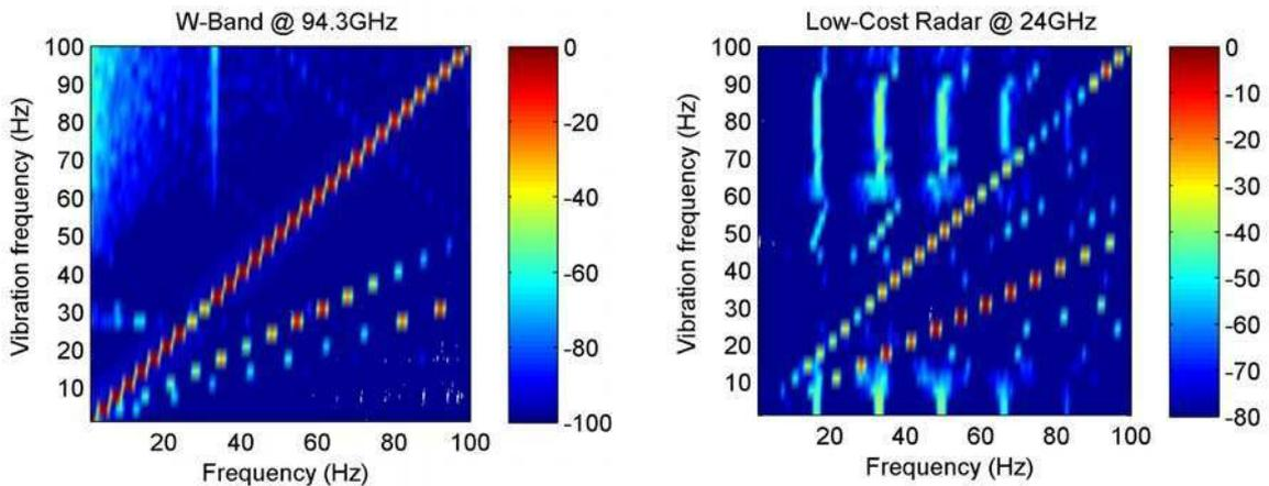
Figure 6: Frequency spectra at vibration frequencies of the shaker system from 1-100 Hz; (left) 94.3 GHz transceiver (right) 24 GHz transceiver. For each vibration frequency also higher harmonics can be seen.
