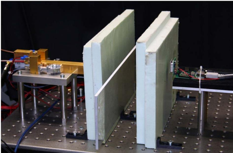
Figure 1: Experimental vibration measurements setup of an aluminum beam behind a barrier material. The laboratory 94.3 GHz system is presented on the left and the low-cost 24 GHz radar sensor on the right side.
