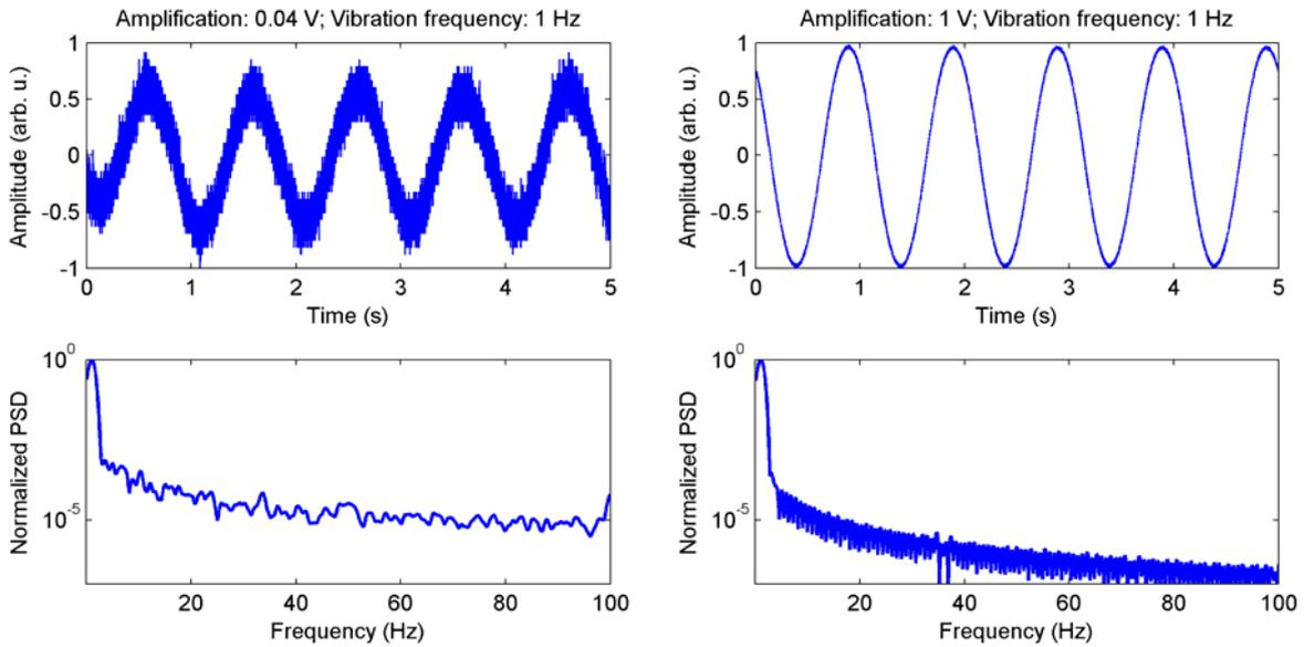
Figure 5: (left) Doppler radar signals for 94.3GHz transceiver at small vibration amplitudes (amplitude of frequency generator: 0.04V) and large vibration amplitudes (amplitude of frequency generator: 1V).
