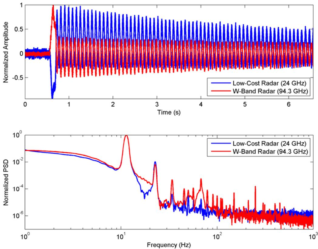
Figure 2: (top) Impulse response in time domain for both transceiver systems; (bottom) Frequency domain representation by means of the normalized power spectral density (PSD). A good agreement was found between the fundamental vibration modes for both frequency bands.
