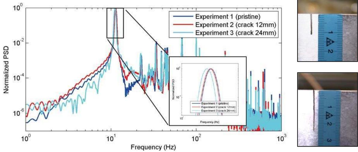
Figure 3: (left) Normalized power spectral density for the pristine and damaged aluminum beam. The crack has a length of 12mm and 24mm, respectively; (right) images of the two considered crack sizes.
