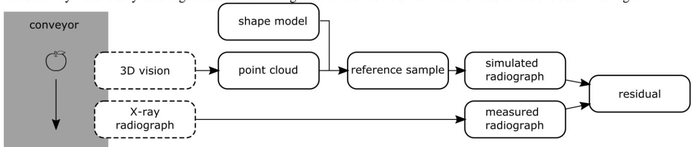
Figure 1: Flowchart of the multisensor inspection method
