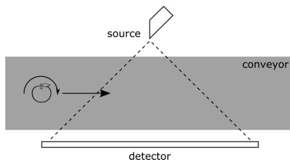
Figure 2: Obtaining projections by using the translation between source and detector and a small rotation of the sample.
