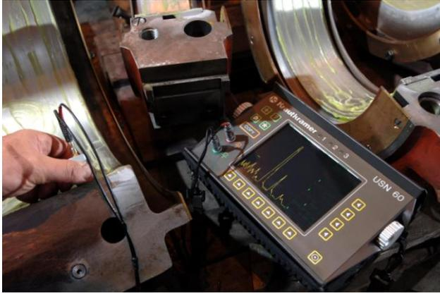
**Figure 1** – Ultrasonic thickness measurement of a simple configuration
