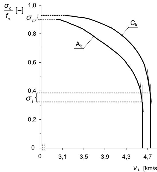
Fig. 4. Longitudinal ultrasonic wave velocity in compressed concretes  $A_k$  and  $C_k$  versus relative stress increment.
