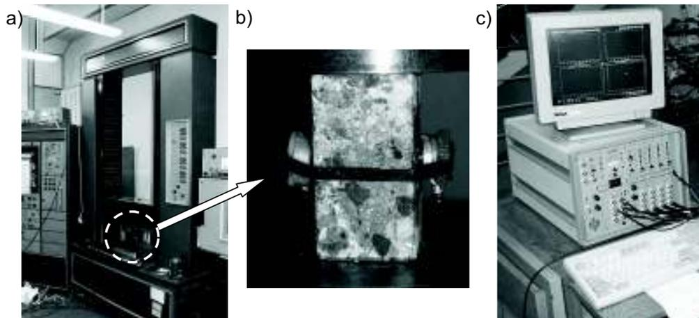
Fig. 1. Stand for measuring acoustic emission in concrete under compression: a) Instron 1126 tester, b) concrete specimen prepared for testing, c) Vallen-Systeme GmbH AMS3 measuring set.
