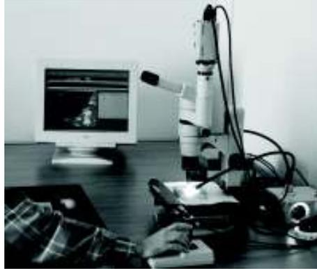
Fig. 2. Setup for investigating air pore structure in hardened concretes.
