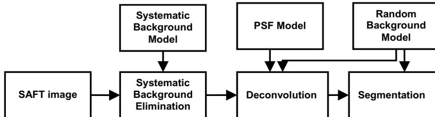
Fig. 2 Block diagram of the defect detection process.
