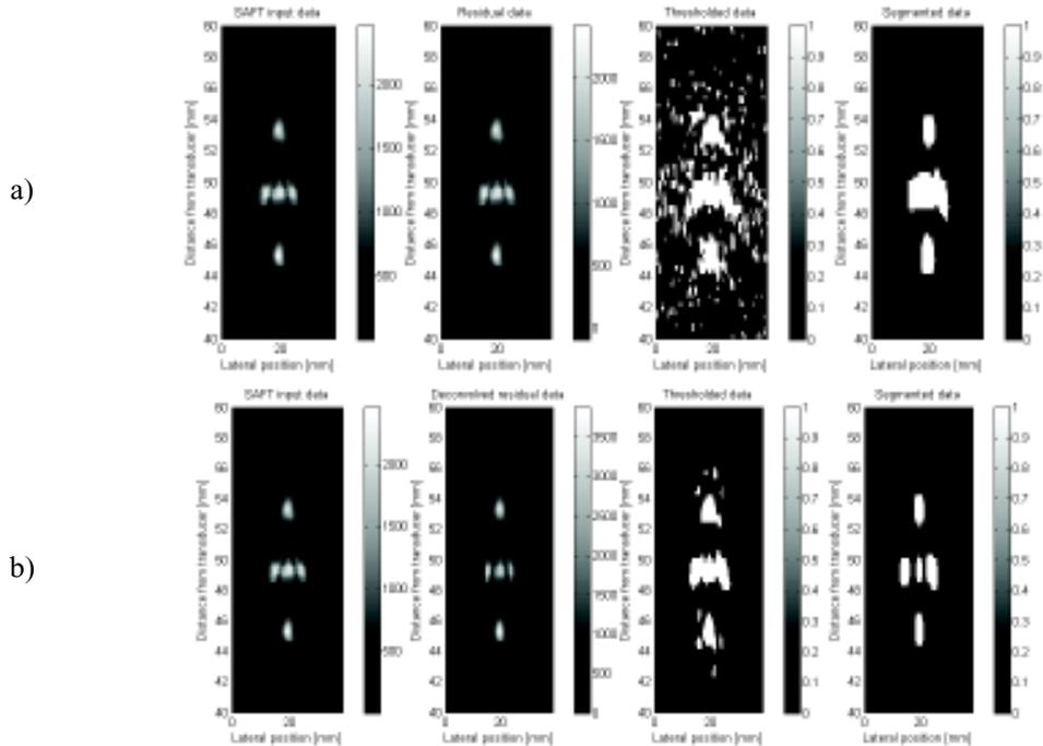
Fig. 4 Results of detection algorithm a) without removal of the convolution distortion, b) using deconvolution.
