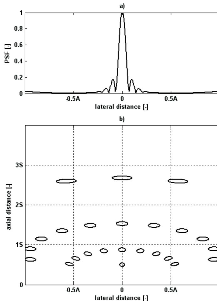
**Fig. 3** Mathematical model of the SAFT PSF ( $A$  ... transducer aperture,  $S$  ... near-field length) – number of transducer elements = 24, element diameter = 1.2mm, pulse frequency = 0.9MHz, ultrasound velocity = 5200m/s
