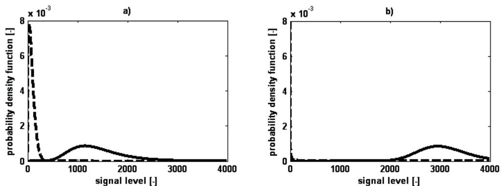
Fig. 5 Histogram of the background noise (dashed line) and defect (solid line) a) before deconvolution, b) after deconvolution.
