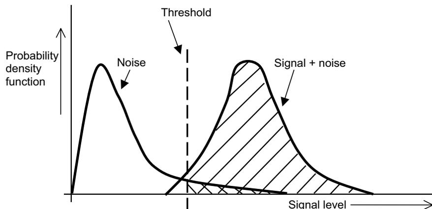
**Fig. 1 Schematic representation of the POD model basis (double hatched area = PFI, double hatched area + hatched area = POD).**
