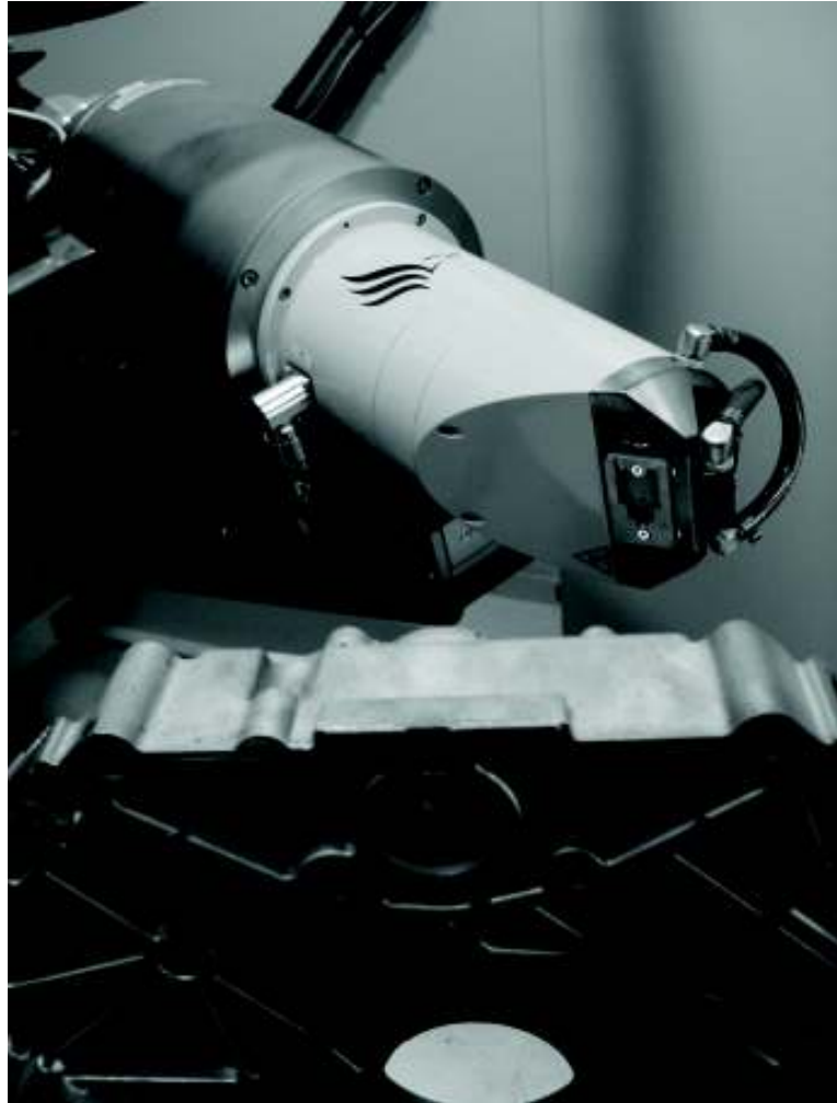
Figure 4: The directional microfocus tube examining a large casting. The cooled reflection target allows for higher energy X-rays to be generated.
