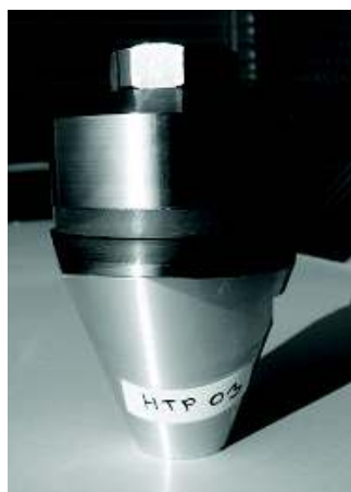
Fig. 3 Piezoceramic power transmitter with mechanical wave concentration
