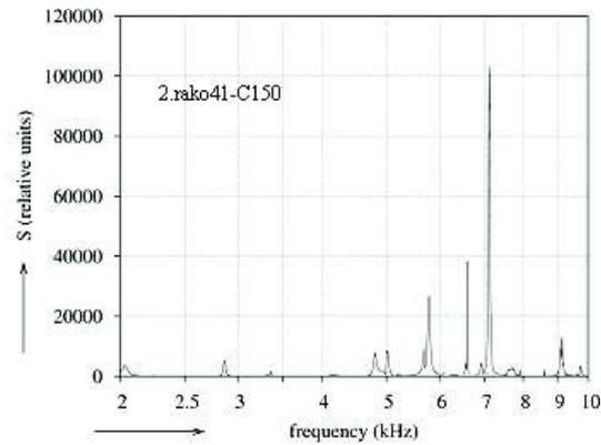
**Fig.2** The power spectral density versus frequency plot for a ceramic tile No. 41 after the 150 freezing and thawing cycles.
