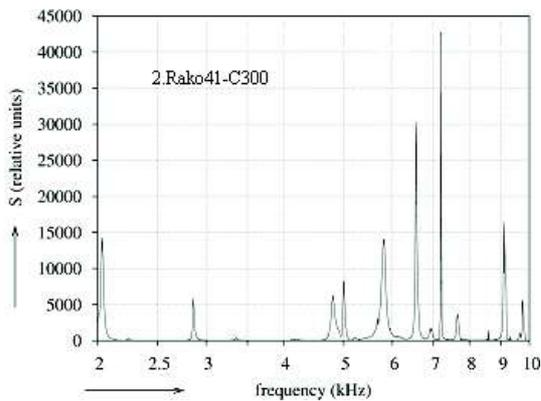
**Fig.3** The power spectral density versus frequency plot for a ceramic tile No.41 after the completion of 300 freezing and thawing cycles.
