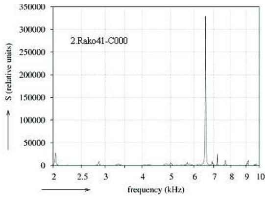
**Fig.1** The power spectral density versus frequency plot for a ceramic tile No.41 before degradation.
