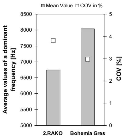
Fig.5: Average values of a dominant frequency after the 150 freezing and thawing cycles: Mean values and variance coefficients
