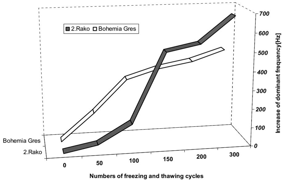
Fig.4 Average incremental values of a dominant frequency versus numbers of freezing and thawing cycles for a ceramic tiles (2. Rako, Bohemia Gres).
