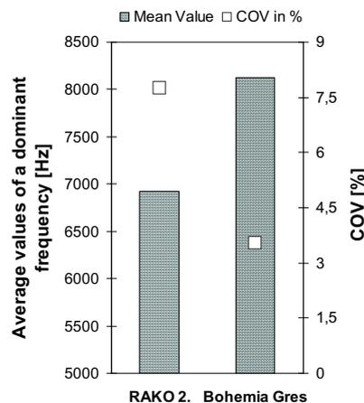
Fig.6: Average values of a dominant frequency after the completion of 300 freezing and thawing cycles: Mean values and variance coefficients
