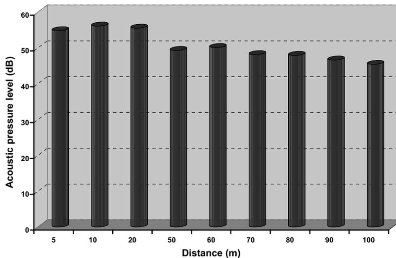
Fig. 2 Diagram of the sound intensity level depending on the distance from the air turbine, measured in the direction opposite to the wheel axis of rotation
