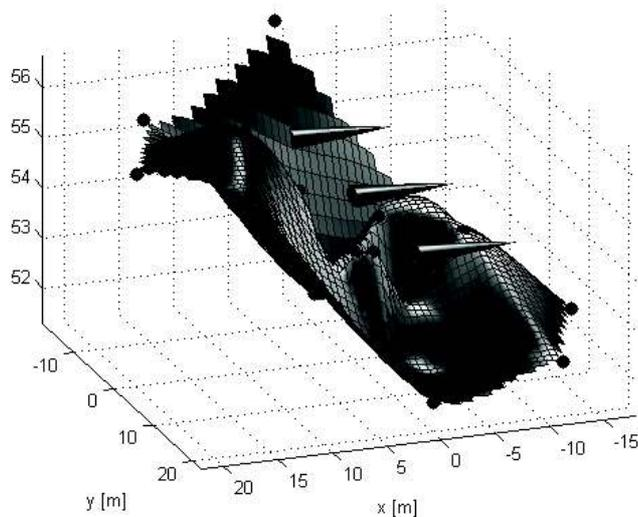
Fig. 6 Spatial distribution of the acoustic pressure level, view from the right side of the air turbine
