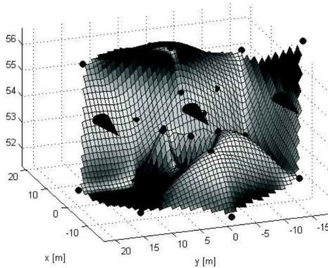
Fig. 4 Spatial distribution of the acoustic pressure level, view from the front of the air turbine
