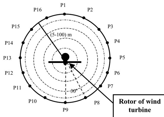
Fig. 1 Distribution of the measurement points around the air turbine
