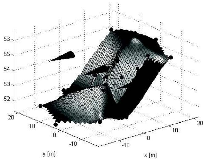
Fig. 5 Spatial distribution of the acoustic pressure level, view from the left side of the air turbine
