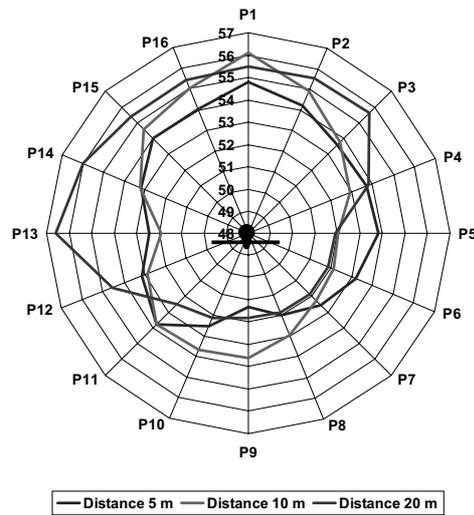
Fig. 3 Circular diagrams showing the acoustic pressure distribution around the air turbine under study for three distance values: 5, 10 and 20 m
