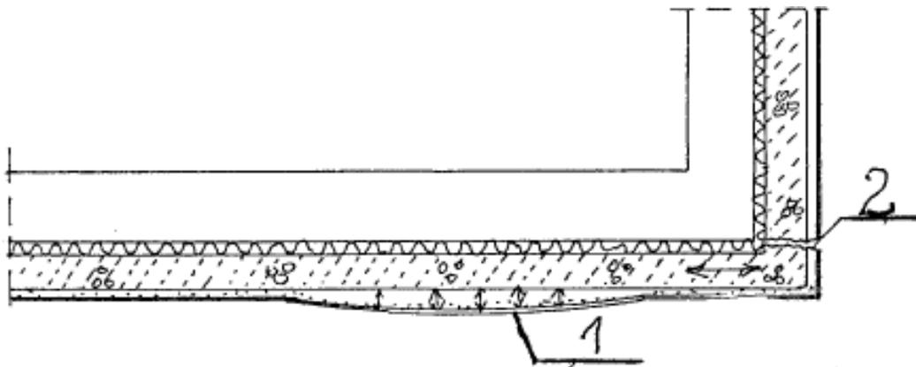
Fig. 5. Damage to plaster caused by plaster elongation relative to still cool base 1 and elongation of gas concrete layer after longer period of heating 2.
