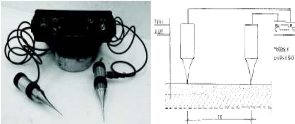
Fig. 4. Measuring equipment and scheme used for plaster tests.
