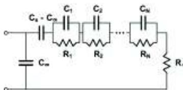
Fig. 4. A series – parallel substitute scheme
