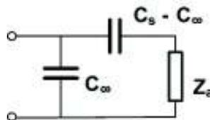
Fig. 2. A substitute scheme for the Cole-Cole model
