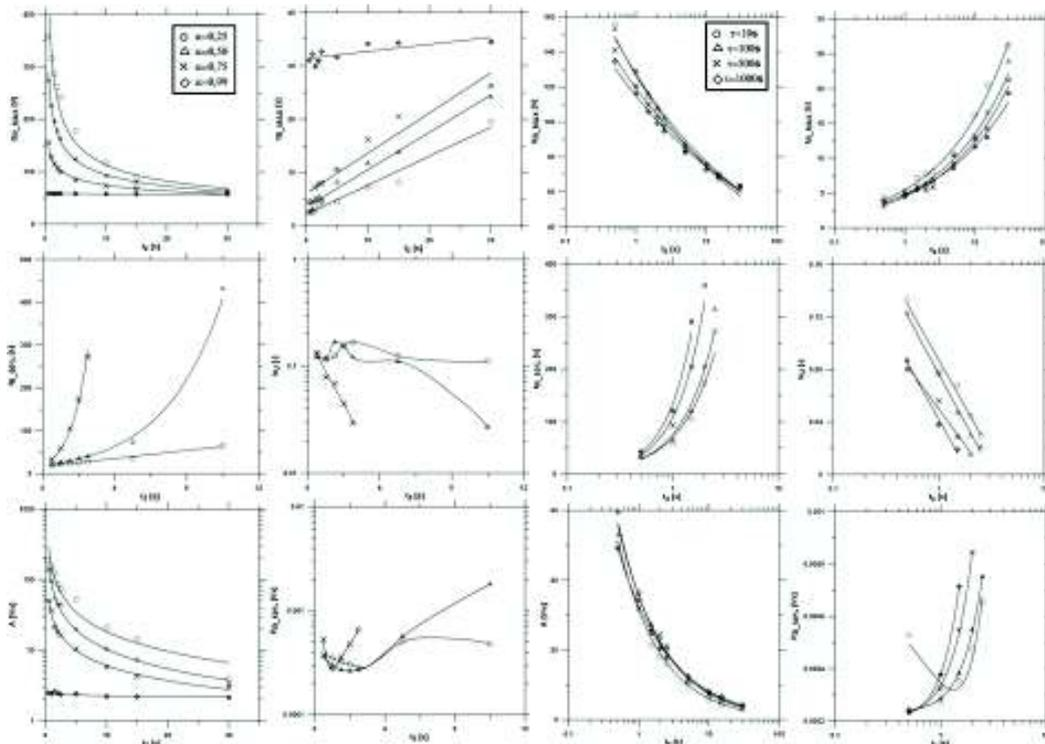
Fig. 7. The influence of parameter  $\alpha$  on the return voltage parameters for a selected relaxation time  $\tau=10s$
