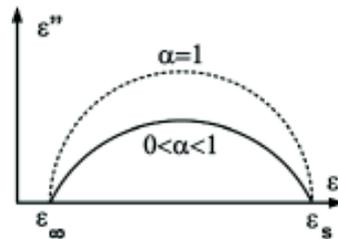
Fig. 1. The Cole-Cole diagram according to equation (2)
