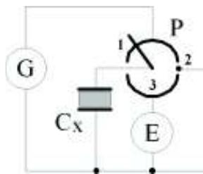
Fig. 5. A diagram of the system for the return voltage measurement
