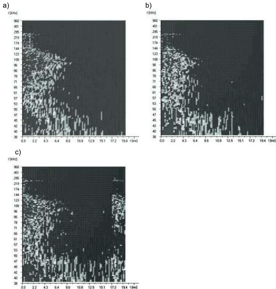
Fig. 3. CWT scaling graphs corresponding to the AE signals generated by PDs:
