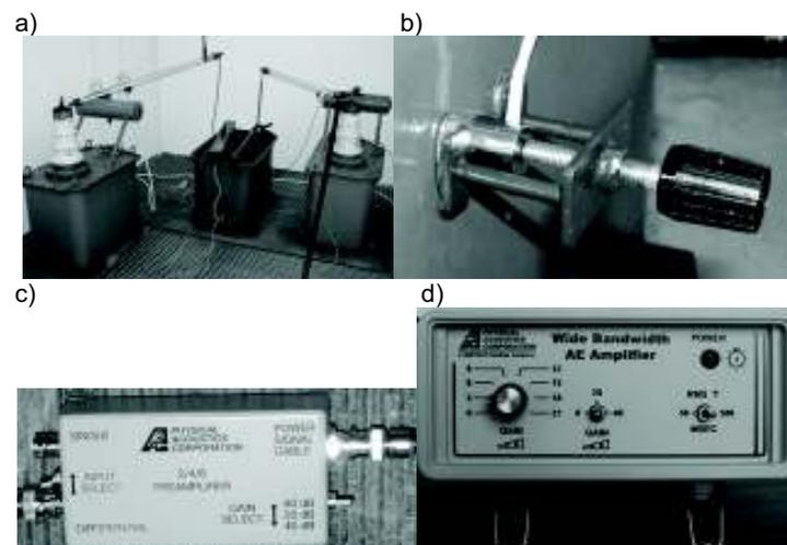
Fig. 2. View of the measuring system : a) measurement chamber, b) piezoelectric transducer, c) subamplifier, d) amplifying and filtering system.
