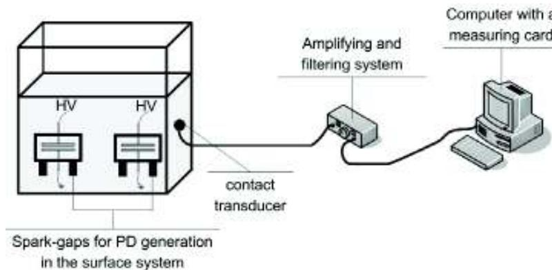
Fig. 1. Diagram of the measuring system
