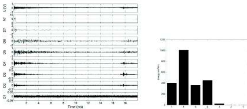
Fig. 4. Discrete wavelet decomposition and the amount of energy transferred by the particular details corresponding to the AE signals generated by PDs:
