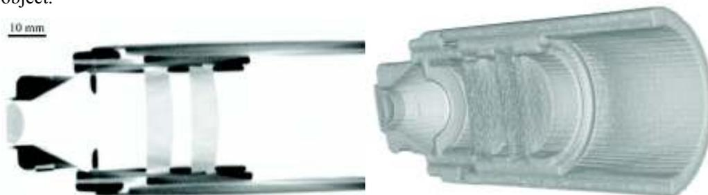
Figure 1. Part of periscope – 2D and 3D model
