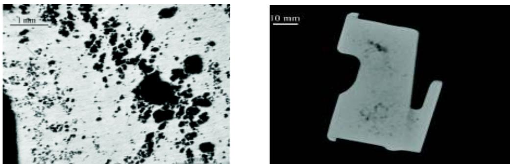
Figure 2. Porosity in zoomed metallographical pattern and cross section of the whole object by means of CT
