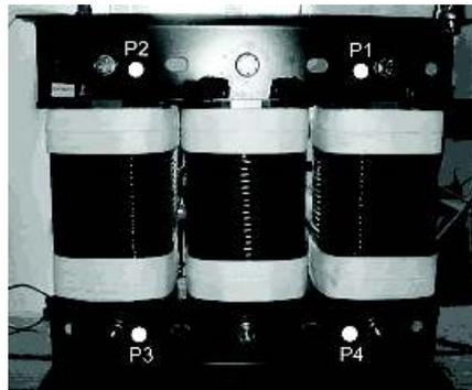
Fig. 1. Low-voltage transformer model under study with marked measurement points
