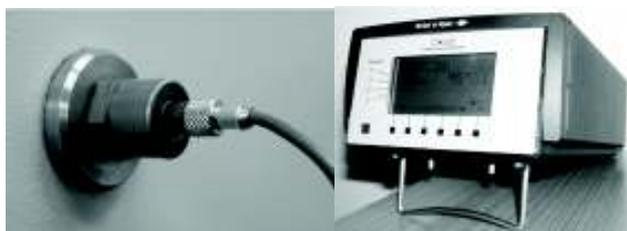
Fig.2. View of the measuring transducer type 752-10, by the firm Endevco and measuring amplifier Nexus 2693, by the firm Brüel & Kjær
