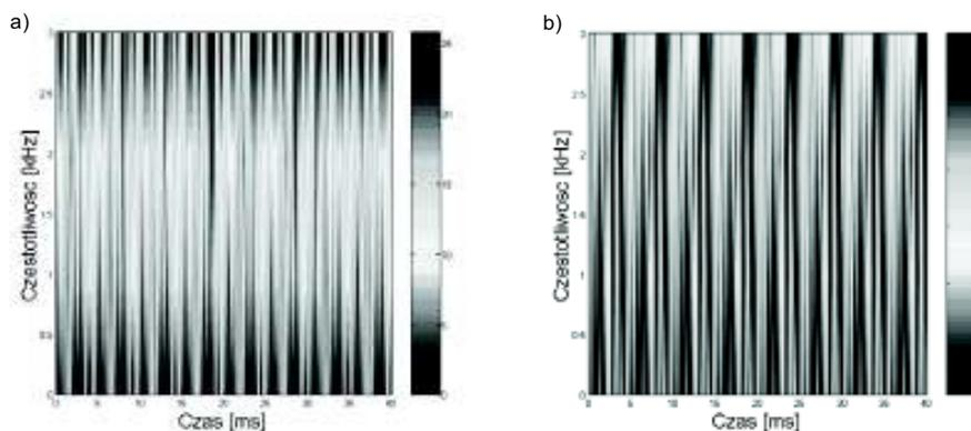
Fig. 4 Two-dimensional spectrograms of power spectral density of vibroacoustic vibrations registered in Point P1 for load 280A;
