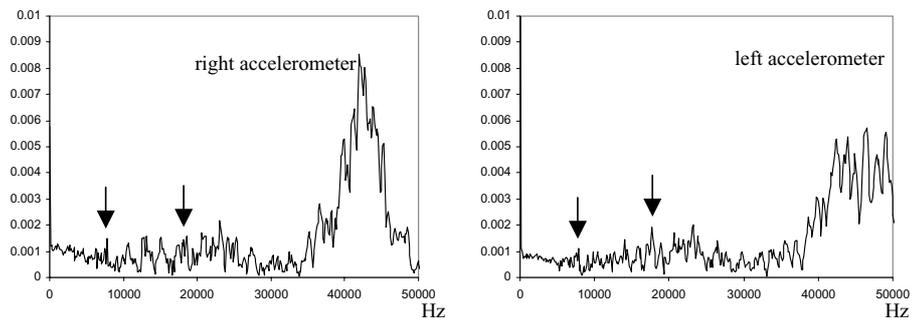
(c) Impact applied at 30 cm where grout was 45 mm
