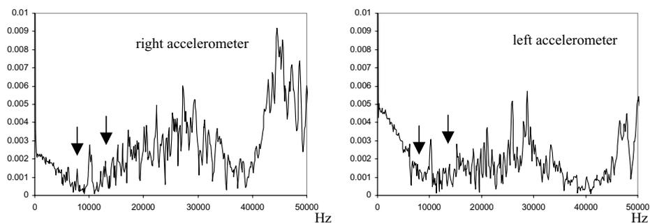
(a) Impact applied at 10 cm where grout was 15 mm
