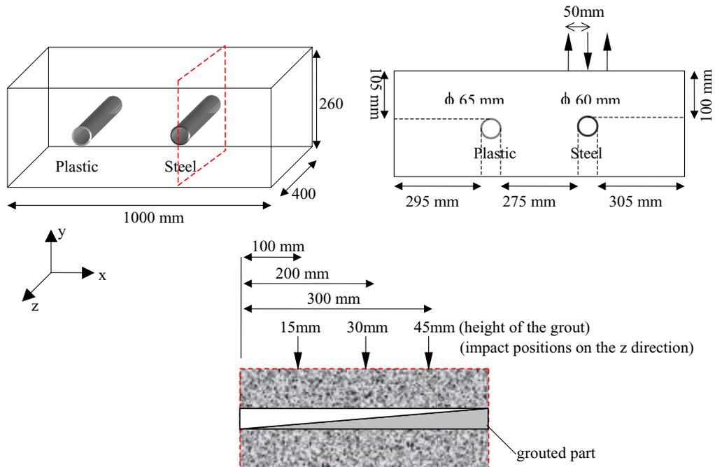
**Figure 2** Concrete specimen tested.
