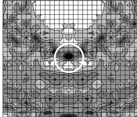
(b) Impact applied at 20 cm where grout was 30 mm
