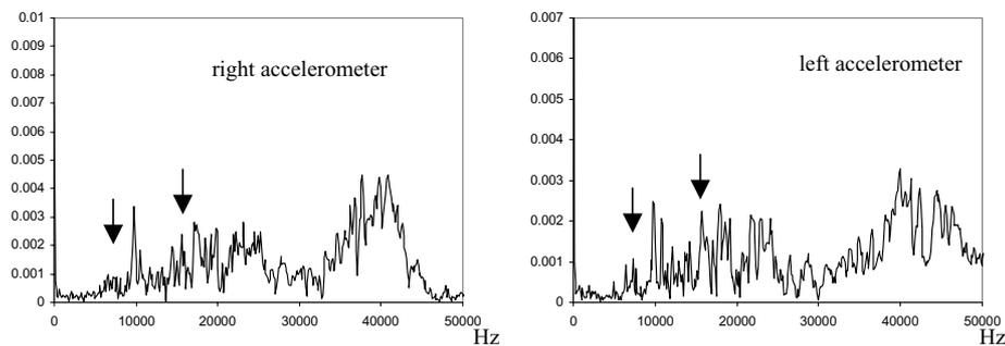
(b) Impact applied at 20 cm where grout was 30 mm
